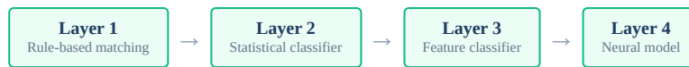
Figure 1: Four-layer pipeline with OR-logic aggregation — any layer flagging triggers detection. Short-circuit optimization skips later layers once a match is found. Total: 23 ms end-to-end, 355 MB RAM, CPU-only.
